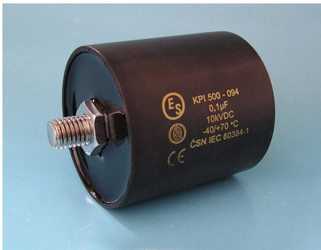
**Dimensions:** D= 63mm, L=65<sup>±1</sup>mm, Lv=13<sup>±1</sup>mm
